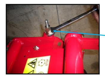
Firstly adjust the contact between the cutting cylinder and the bottom blade to achieve the best cut possible keeping the contact even across the entire width of the blades.
