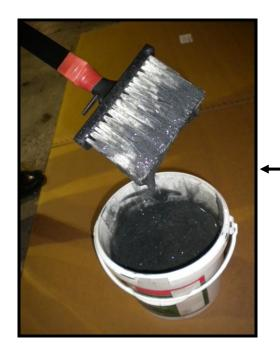
Dip the long handled brush into the back-lapping paste until the brush has a good covering of the abrasive paste.
