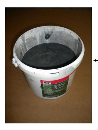
A pot of back-lapping paste. Back-lapping paste is a water soluble abrasive grinding paste.
