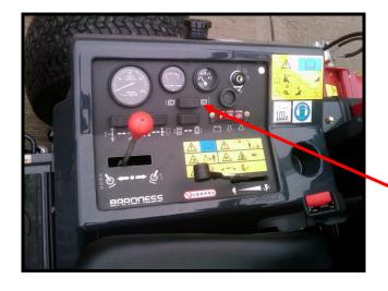
With the aid of an assistant and with the parking brake on, start the engine and leave it running at idle. The assistant should remain on the seat and able to stop the machine in an emergency.
