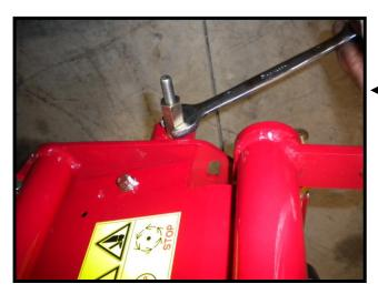
Normally after back-lapping, no further adjustments are necessary, however, you might need to readjust the cut slightly by bring the cylinder down onto the bottom blade using the adjusters as shown.
