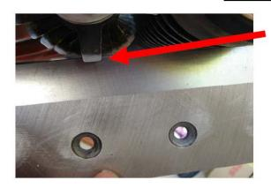
Typical De-Thatching height set is **0.100" to 0.120" <u>BELOW</u>** the **<u>Roller Height</u>** depending on the green and soil conditions.
