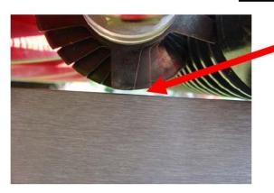
Typical Groomer height set is between 0.040" to 0.060" <u>ABOVE</u> the <u>Roller Height</u> depending on the green and soil conditions.
