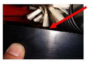
Typical Rotary Brush height set is the same as <u>Height of Cut</u>. In this photo, the cutting height is set at 0.150".
