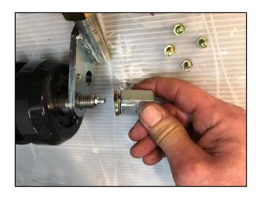
On one end of the roller, remove the roller retaining nut as shown.
