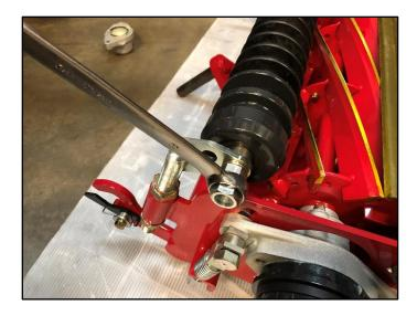
Slacken, but do not remove, both front roller nuts.
