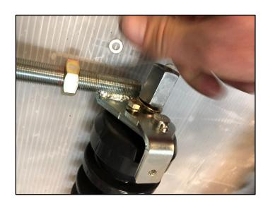
Loosely fit the front roller nuts to both ends of the roller. Do not tighten them at this stage.
