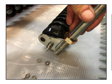
Remove the roller bracket from the axle shaft of the front roller.
