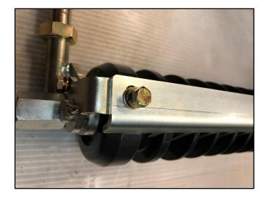
Fit the scraper bar to the new scraper brackets as shown using the provided M6 bolts, washers and spring washers. Do not tighten them at this stage.
