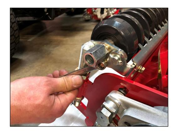
LM331 Tees and Approach Mower Fitting Front Roller Scrapers
